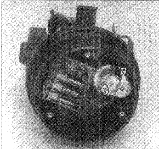
Fig. 4: Showing three AA-size batteries installed inside the drive base.
